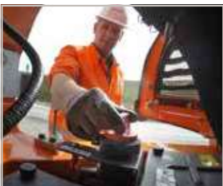
Battery cut-off switch
