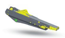
No matter what the application is, the 570T can be configured to properly address every need. The optional Extendable Dipper and auxiliary hydraulics allow to reach a digging depth of 5.6 meters and fit a hammer for demolition application.
