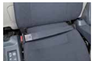
● Retractable seatbelt requires no manual adjustment
