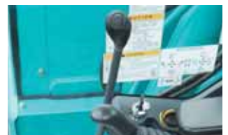
●Travel speed select switch ※The switch is equipped with the dozer lever. (Option)
