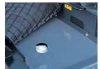
Washer fluid tank located under the cab floor mat.
