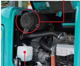
Radiator reservoir tank
