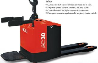
Side-loaded battery EPS AC Steering automatic deceleration
