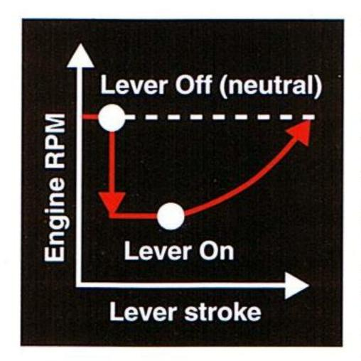
When the control lever is placed in neutral, engine speed is automatically lowered to save fuel, reduce the noise level and
