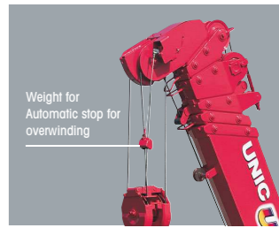
8 Automatic stop for overwinding
