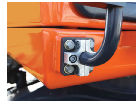
New handrail & guardrail The new fittings are now ISO 2867:2007 compliant. Access is facilitated and the fittings have been strongly reinforced.
