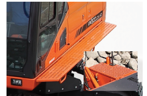
Cat walk (platform) as standard on DX480LCA-HD & DX500LCA-HD Larger anti-slip surface on the upper structure for more safety.
