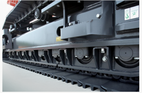
Full track guard & Full heavy-duty undercarriage parts
