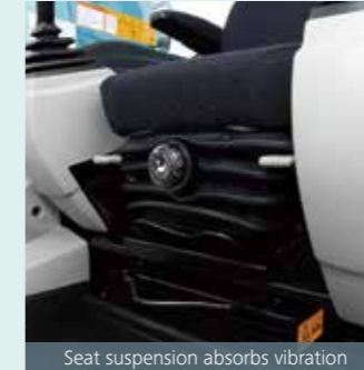
Seat suspension absorbs vibration
