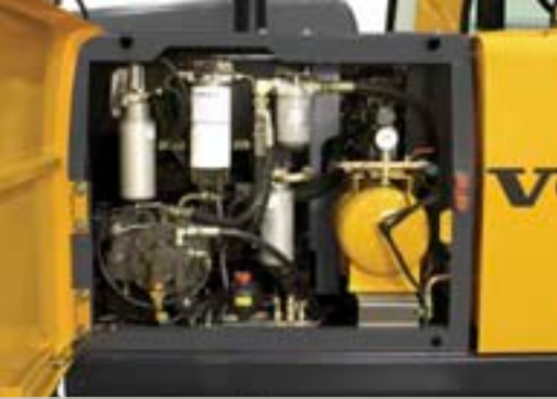
• Easy access for hydraulic pump filters.
