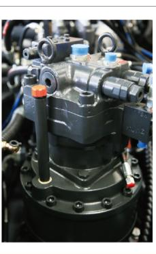
High-efficiency large-displacement motor, the rotary motor increases the displacement and increases the rotary torque of the whole machine by 12.1%
