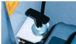
Engine cable throttle used when CPU is down
