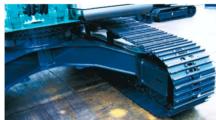
New design of crawler frame
