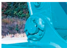
New bucket-clatter adjustment mechanism
