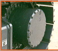
Stronger casing for travel motor
