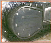
Reinforced travel motor cover
